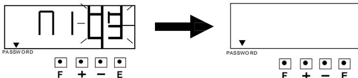
3. After you finished setting the password, press the [E] button again, the LCD screen will return to normal mode.
