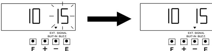
4. After you finished setting the external signal / built buzzer, press the [E] button again,
