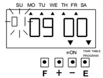
After you finished confirming the program, press the [E] button four times, the LCD screen will return to normal mode.
