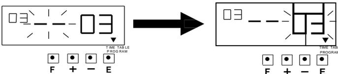
3. Press the [+] or [-] button to set at “--”, and then press the [E] button, the display changes to the following figure.
