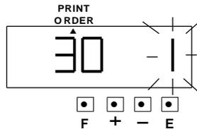
Such as example, press the [+] or [-] button to set at “1” and press [E] button, at the same time the LCD screen only display “▲” under the “Print Order” mark.
