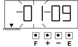
2. Press the [+] or [-] button to set the first two digits at [--], and then press [E] button. The display changes to the following figure.
