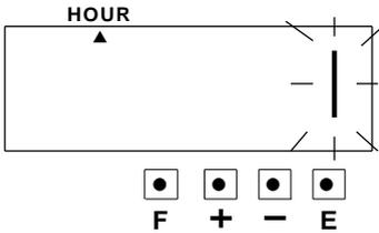
3. If you want to set another function, press the [F] button to continue setting. If you finished setting the functions, press the [E] button again. The LCD screen will return to normal mode.
