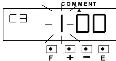
Such as example, the 1st character is "L", press the [+] or [-] button set at "0d", and press the [E] button.
