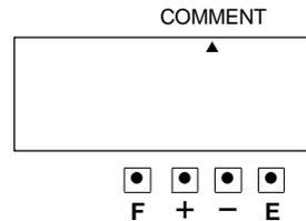
2. If you want to set another function, press the [F] button to continue setting. If you finished setting the functions, press the [E] button again. The LCD screen will return to normal mode.
